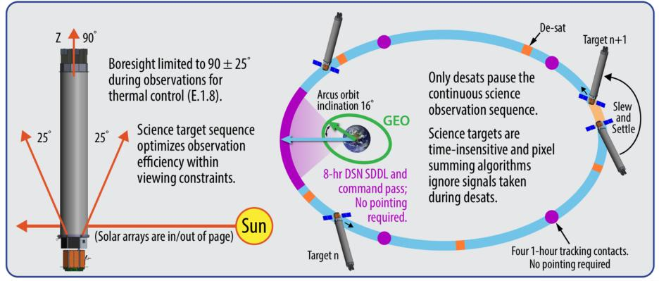
Lunar resonant orbit offers infrequent eclipses, a stable thermal environment, and long-term orbit stability that enables simple operations.
