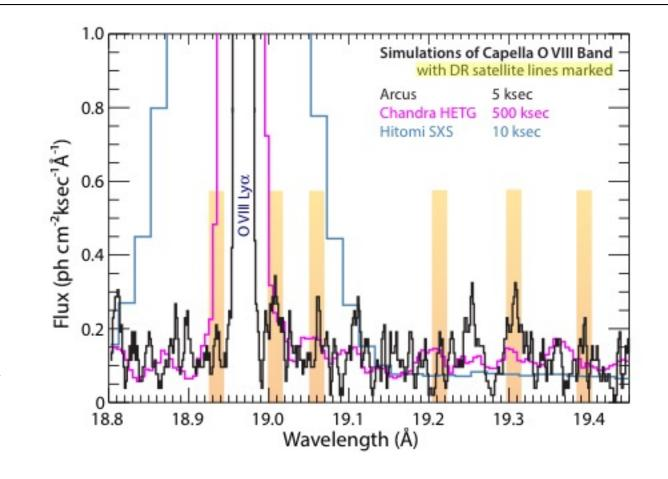
Chandra HETG is limited by resolution and throughput, and a microcalorimeter like Hitomi cannot resolve the features.
